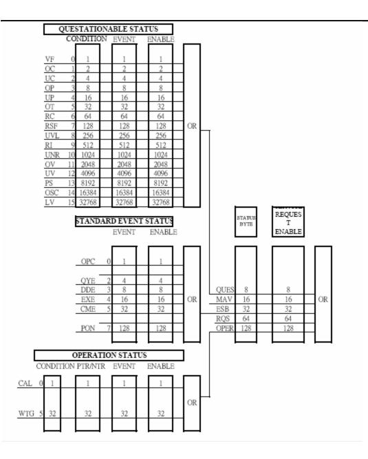
and Operation Event registers to cause the following actions. This command is not channel specific, it applies to the entire mainframe.
