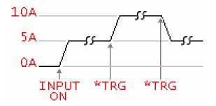
MODE CURRent or MODe:CURRent TRIGger:SOURce BUS TRANsient:MODE TOGGIe CURRent 5 CURRent:TLEVel 10 INPut ON TRANsient ON
