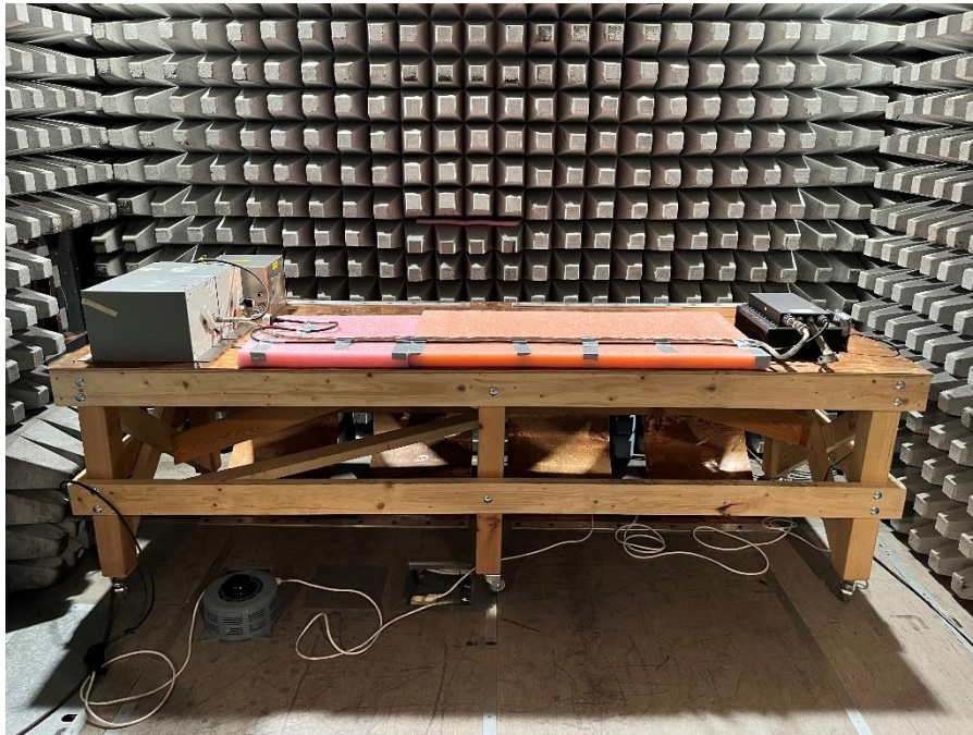
Fig. 17.10 MIL-STD-461F CE102 and RE102 test set-up
