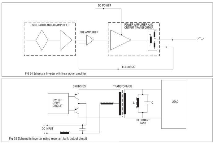
tank. At the resonant frequency the tank represents a very low impedance source to the load so has good capability to cope with dynamic and non-linear loads. Leading and lagging power factors are handled with equal ease.
