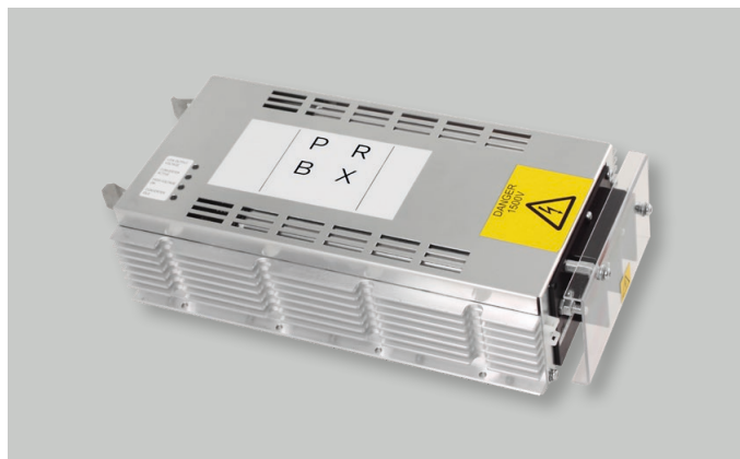
Figure 02 – Low Battery Voltage Starter are connected to high voltage catenaries to deliver a low battery voltage, requiring very high insulation and high-level safety constraints
