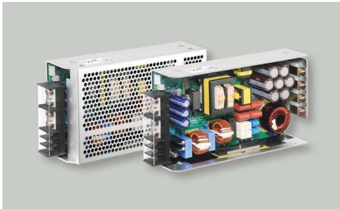
Figure 05 – COSEL power supply with multi-modes for voltage or current constant from max to near zero (Source PRBX/COSEL)
