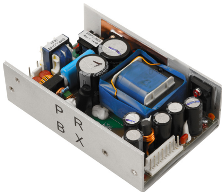
Figure 04 – One step conversion 225W power supply (Powerbox OFM 225) based on One Step Conversion technology.
