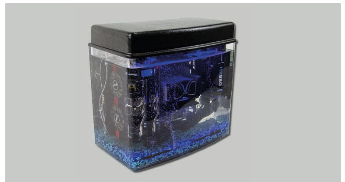
Illustration 01 – Mineral oil cooled PC (Picture: PRBX / Courtesy of Puget System)
