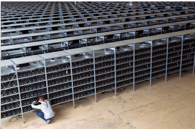
Illustration 02 – KnC Miner 10 megawatt data center filled with high-powered computers mining for cryptocurrency in Boden (Sweden) (Picture: PRBX / KnC Miner-2014)
