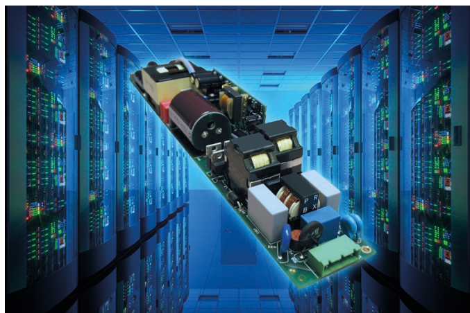
Illustration 07 – PRBX AC/DC power supply OFI600A-12 designed for immersion cooling applications (Picture: Powerbox (PRBX))
