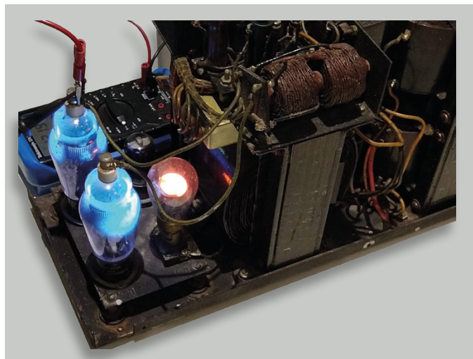
Figure 01 – Thyatron power supply REC-30 for the teletype Model 19 used in the naval communications system in 1940s
