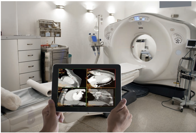
Figure 06 – MRI equipment with advanced data acquisition requires very stable power supplies able to operate in high magnetic field.
