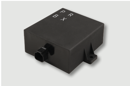
Rugged DC/DC Booster for Marine diesels engine delivering constant voltage to the engine monitoring system during startup. The unit generates boosted voltage to compensate lower battery voltage during the ignition phase.
