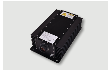
Dual channel 2x27 VDC/10A DC/DC converter for Marine engine control. Typically used for safety equipment requiring redundant power sources, when redundancy is not required but the application requires two independent outputs, the ENMA500D24/2x27-CC offers two 27VDC fully isolated outputs.
