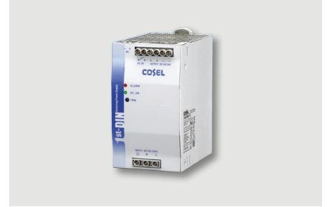
KHEA/KHNA480 Series 480W Din-rail power supply In: 85-264VAC Out: 24VDC/20A (peak 30A) DNV/GL certificate
