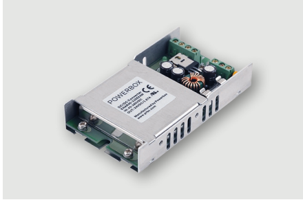
Railway line 20 and 40 ENAR20W Series ENAR40W Series 20W or 40W 4:1 inputs for all EN55150 voltages DC/DC converter"
