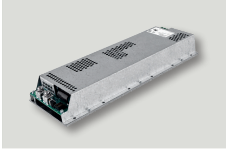
Defense line OFD AC 1200W, Enclosed, rugged design AC/DC switch mode power supply 85-264VAC input with PFC Isolated output
