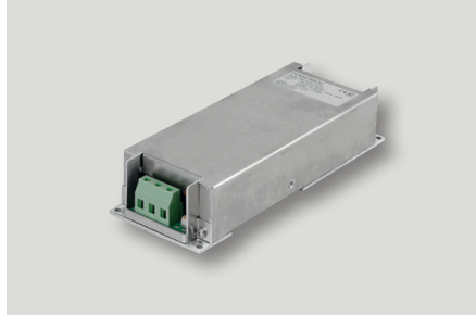
Defense line 150 AC 150W, Enclosed, rugged design AC/DC switch mode power supply 85-264VAC input with PFC Isolated output
