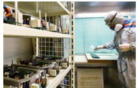
Varnishing at our specialized service partner in Germany
