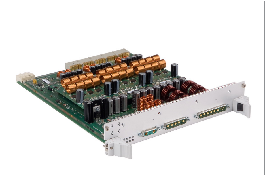
Three phase coreless power supply using three GB350 modules
